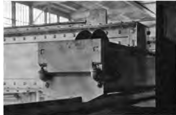
Fig. 4. Bumper on Crane Carriage, and Guard in Front of Track Wheel.*
